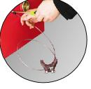
Optional certified antistatic device: Securely connects grounding to safety cabinet, preventing fire from static sparks.
