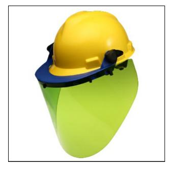
High Performance Arc Flash Protective Face Shield Kit for electricians based on the PAULSON Nanotechnology. Includes cap bracket with US clips. With Premium Coating. Tested to an ATPV of 8 cal/cm2 as per ASTM F2178 (Open Arc Test). Meets NFPA 70E (HRC 2). Patented product.
